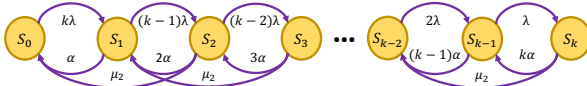
Fig. 2: The transition rate diagram of the Markov chain determined by the bipartite policy \pi^B .
